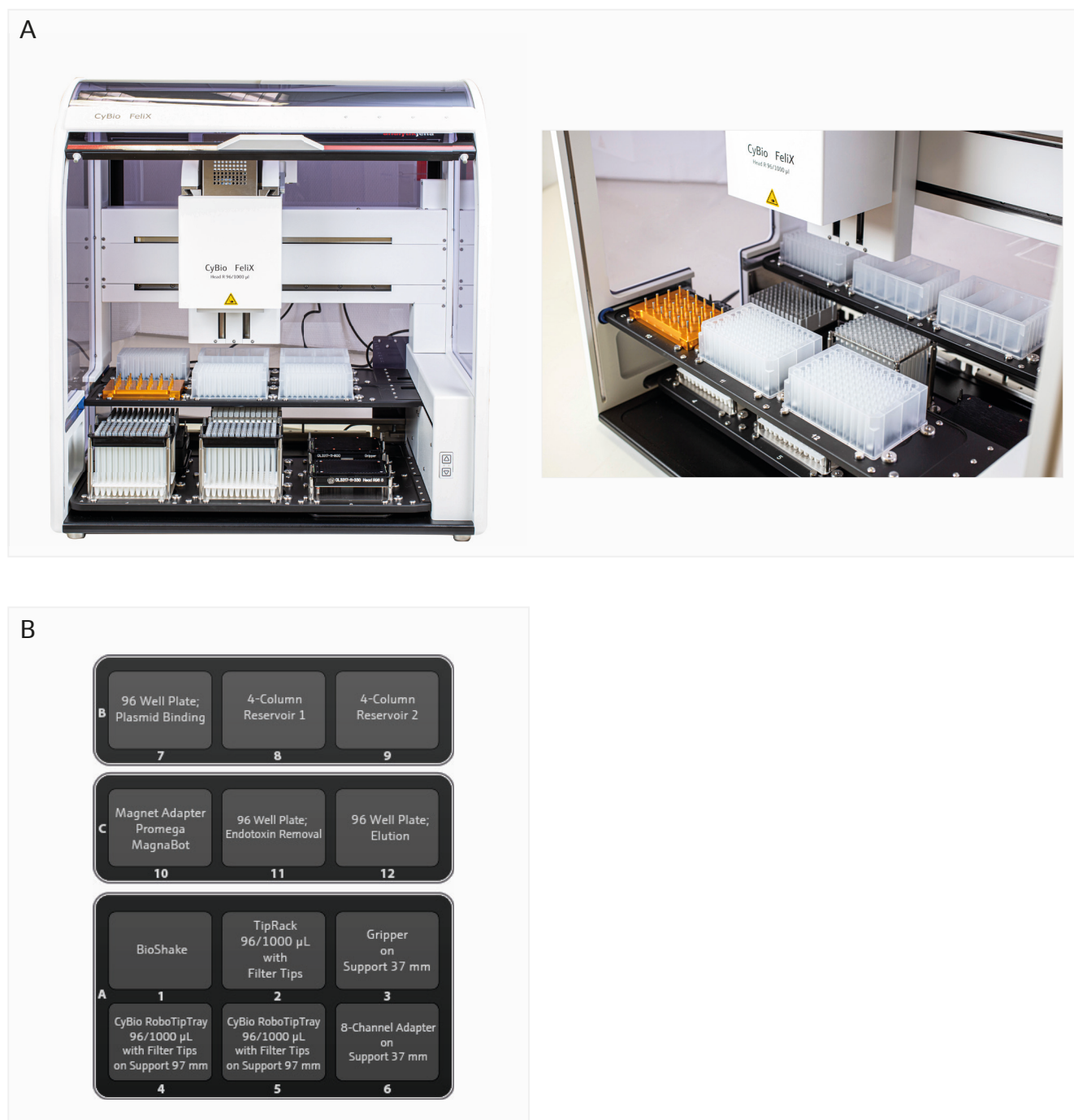
Figure 1: Deck layout for plasmid DNA purification on the CyBio FeliX Liquid Handler using the Wizard MagneSil Tfx™ System.
