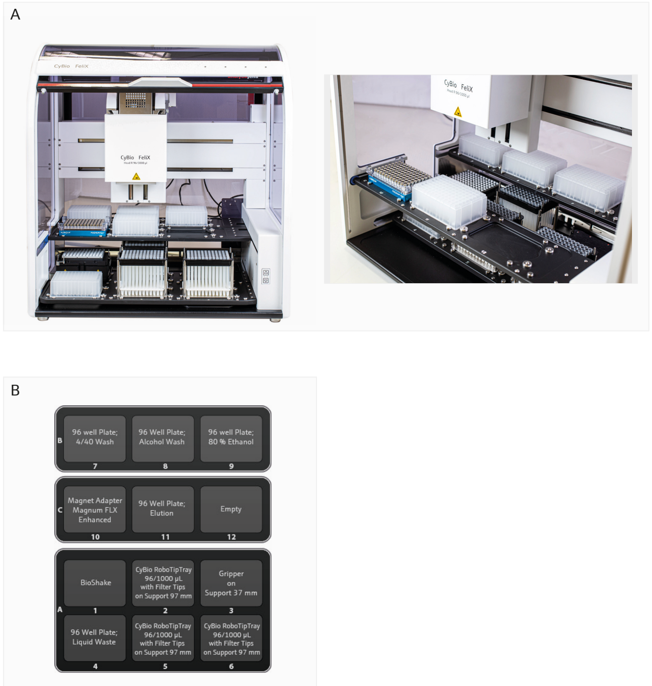
Figure 1: Deck layout for the Maxwell® HT Viral Total Nucleic Acid Kit on the CyBio Felix Liquid Handler.
