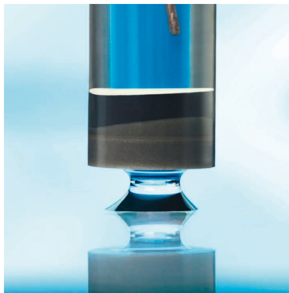
Figure 2: Drop measurement with an InLab Surface
