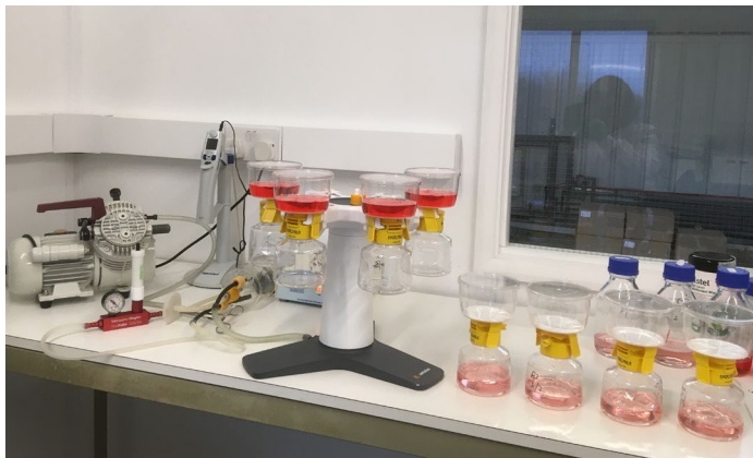
Figure 1: Experimental Setup for Filtration of Challenge Suspension
