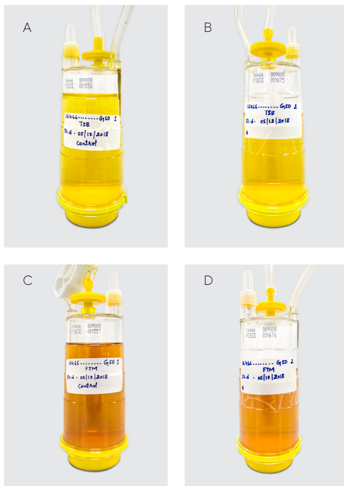
Figure 1: No microbial contamination after repeated sample extraction. Representative images of the Sterisart® 16466 GSD version filled with TSB (A and B) FTM (C and D) incubated for 24 days at 22.5° C and 32.5° C respectively. Negative controls are shown in A and C. Canisters in B and D were pierced 102 times for sample extraction.
