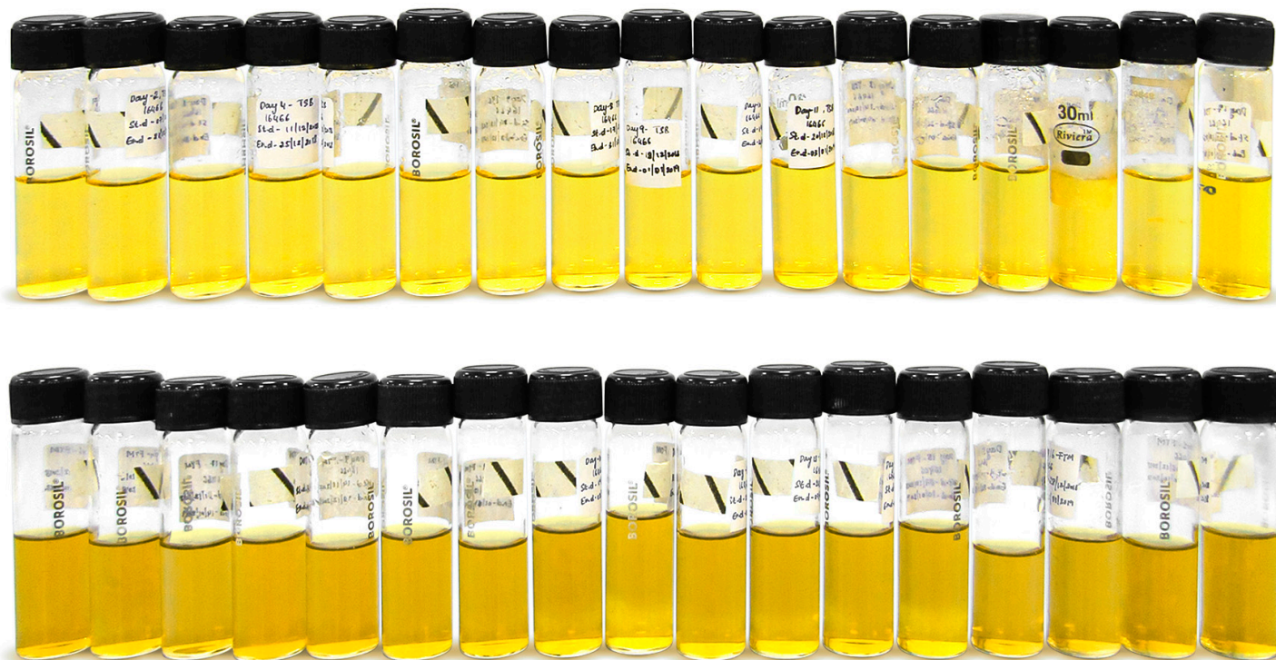
Figure 2: No microbial contamination in samples extracted from Sterisart® 16466 GSD after incubation in glass vials. Samples were inoculated into glass vials containing TSB (upper panel) and FTM (lower panel) were grown at 22.5° C and 32.5° C, respectively, for 14 days.
